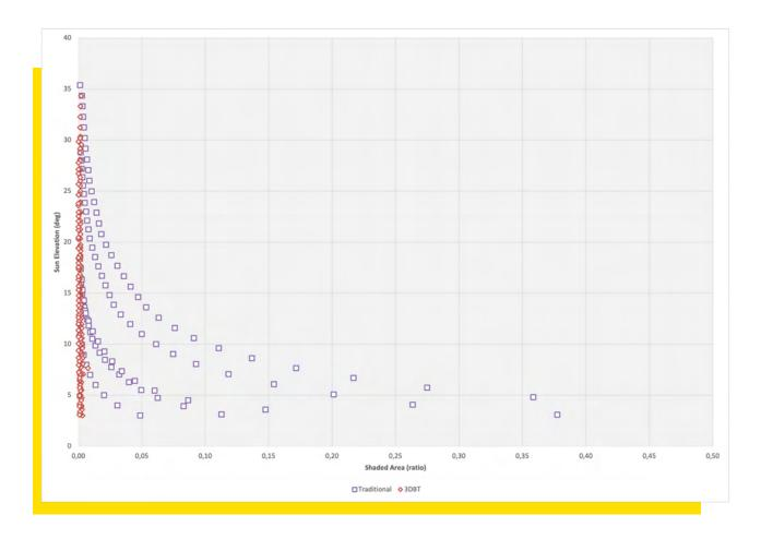
The red points represent the ratio of shaded area against the sun's elevation using a traditional backtracking algorithm. The more red points along the x axis, the more panels that are shaded.
